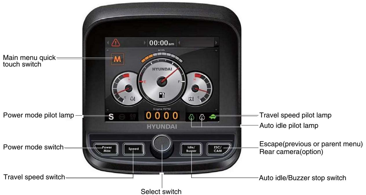
※ When the switches are selected, the pilot lamps are displayed on the LCD. Refer to the page 3-10 for details.
